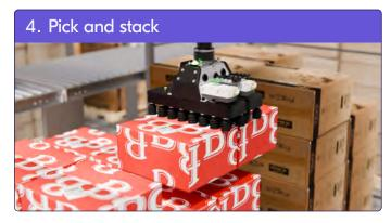
Items are picked with a suction based gripper and are directly transferred to the correct pallet respecting constraints such as barcodes facing out.
