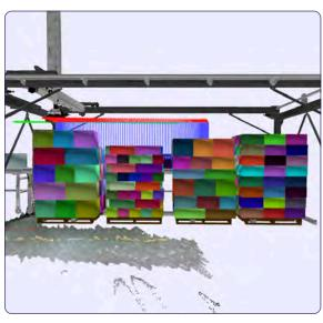
When pallet stacking patterns need to be controlled, AmbiStack can use customer defined stacking patterns from an item master to stack goods.
