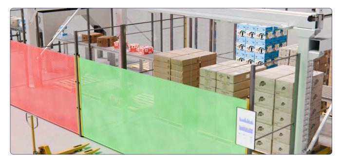
Light curtain guarded safety zones allow operators to remove and replenish pallet positions in one half of the machine, while the gantry continues to stack in the other.
