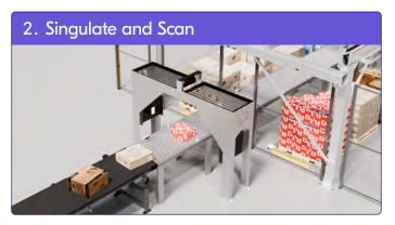
Items are separated so they can be scanned and dimensioned in the scan tunnel.
