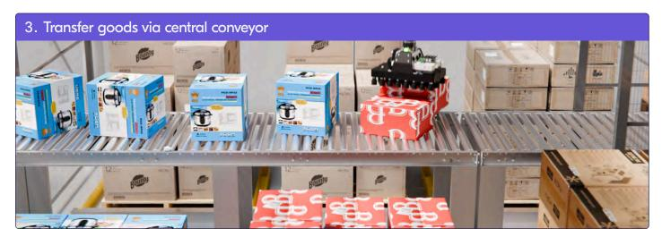
Conveyance transfers goods close to the pallets being actively sorted to optimize palletizing speed.
