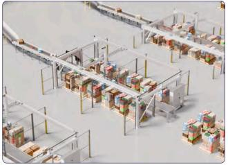
Connect AmbiStack to existing conveyance used to transfer goods from trailer unload. The AmbiStack solution takes over right before the optional scan tunnel.
