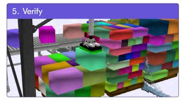
Machine vision ensures that all items are densely stacked in the correct position and that pallet integrity is maintained.
